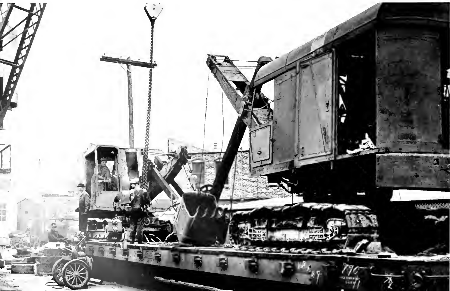
Two big power shovels transported to Sacramento Highway Shops by freight car for extensive repairs, replacements and overhauling
